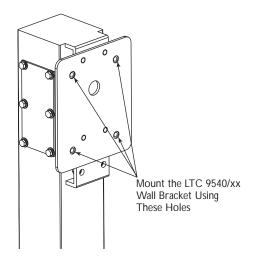
Figure 11 Mounting the LTC 9540/xx Wall Bracket
